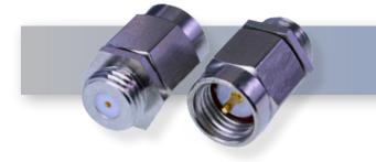
The 500285 is an SMA Male thread-in field replaceable connector by HASCO. This SMA Male accepts a 0.020" Pin Diameter and will operate up to 27 GHz. Thread-In connectors can be directly mounted on component housings with the use of a hermetic seal or launch pin.
