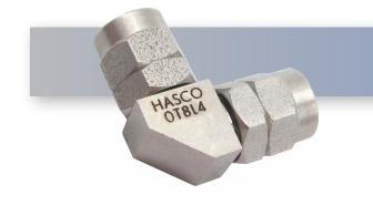
The HASCO **185P-185P-RA** is a 1.85mm Male to 1.85mm Male in-series adapter from HASCO. This in-series 1.85mm to 1.85mm right angle coax adapter will operate up to 67 GHz. Adapters that have a male to female or plug to jack configuration are known as "connector savers." Typically, a low loss or low VSWR male to female adapter is placed on more expensive component connectors to prevent damage.
