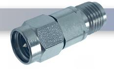
The HASCO **24J-SMAP-FM** is a 2.4mm Female to SMA Male between series adapter manufactured by HASCO Components. This between series 2.4mm to SMA coax adapter will operate up to 26.5 GHz. Adapters that have a male to female or plug to jack configuration are known as "connector savers."
