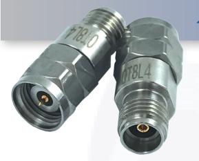
The HASCO **24P-35J-MF** is an Adapter that operates from DC to 33 GHz and handles up to 1,000 cycles. Our 2.4mm to 3.5mm Between-Series Adapters offer 1.15:1 max VSWR.
