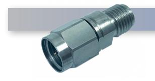
The HASCO **24P-SMAJ-MF** is a 2.4mm Male to SMA Female between series adapter manufactured by HASCO Components. This between series 2.4mm to SMA coax adapter will operate up to 26.5 GHz. Adapters that have a male to female or plug to jack configuration are known as "connector savers."
