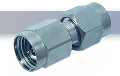
The HASCO **24P-SMAP-MM** is a 2.4mm Male to SMA Male between series adapter manufactured by HASCO Components. This between series 2.4mm to SMA coax adapter will operate up to 26.5 GHz. Adapters that have a male to female or plug to jack configuration are known as "connector savers."
