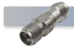
The HASCO **29J-185J-FF** is a Precision Between-Series RF Adapter that operates from DC to 40 GHz. and offers 1.15:1 max VSWR.
