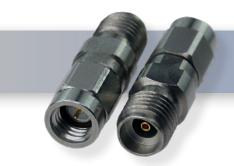
The HASCO **HAD-29J-SSMAP** is a general purpose 2.92mm Female to SSMA Male between-series adapter from HASCO. This between-series coaxial adapter will operate up to 40 GHz. The 2.92mm connector mates mechanically with commercially available SMA and 3.5mm connectors.
