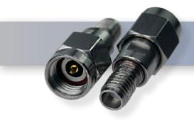
The HASCO **HAD-29P-SSMAJ** is a general purpose 2.92mm Male to SSMA Female between-series adapter from HASCO. This between-series coaxial adapter will operate up to 40 GHz. The 2.92mm connector mates mechanically with commercially available SMA and 3.5mm connectors.
