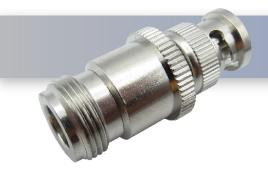
The HASCO **HAD-BNCP-NJ** is a general purpose BNC Male to N Female between-series adapter from HASCO. This between-series coaxial adapter will operate up to 4 GHz.
