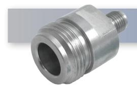
The HASCO **NJ-SMAJ-FF** is a Type N Female to SMA Female Straight RF Adapter that operates from DC to 18 GHz. and offers 1.25:1 max VSWR.
