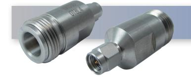
The HASCO **NJ-SMAP-FM-01** is a Type N Female to SMA Male Straight RF Precision Adapter that operates from DC to 18 GHz. and offers 1.15:1 max VSWR.
