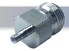
The HASCO SMBJ-NJ-MF is an RF Push-On Between Series Adapter that operates from DC to 6 GHz and handles a minimum of 500 mating cycles. Our SMB to N Type Adapters offer 1.20:1 max VSWR.
