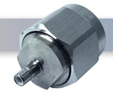
The HASCO SMBJ-NP-MM is an RF Push-On Between Series Adapter that operates from DC to 6 GHz and handles a minimum of 500 mating cycles. Our SMB to N Type Adapters offer 1.20:1 max VSWR.
