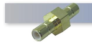
The HASCO SMBJ-SMBJ-MM is an RF Push-On Adapter that operates from DC to 6 GHz and handles a minimum of 500 mating cycles. Our SMB Adapters offer 1.20:1 max VSWR.
