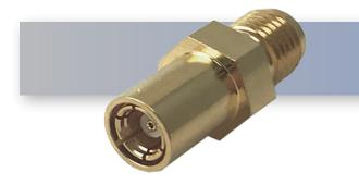
The HASCO SMBP-SMAJ-FF is an RF Push-On Adapter that operates from DC to 6 GHz and handles a minimum of 500 mating cycles. Our SMB to SMA Adapters offer 1.20:1 max VSWR.
