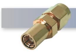
The HASCO SMBP-SMAP-FM is an RF Push-On Between Series Adapter that operates from DC to 6 GHz and handles a minimum of 500 mating cycles. Our SMB to SMA Adapters offer 1.20:1 max VSWR.
