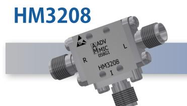
The Advanced Microwave HM3208 is a double-balanced 18 to 32 GHz microwave mixer with an IF frequency range of DC to 8 GHz. The LO is driven with +14 to +17 dBm, and as an up or downconverter features typical conversion loss of 9 dB, L to I isolation of 23 dB, and L to R isolation of 32 dB. Maximum Input power is +20dBm.
