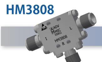
The Advanced Microwave HM3808 is a double-balanced 18 to 38 GHz microwave mixer with an IF frequency range of DC to 20 GHz. The LO level is driven with +15 to +18 dBm, and typical conversion loss of 10 dB, L to I isolation of 30 dB, and L to R isolation of 26 dB. Maximum Input power is +20dBm.
