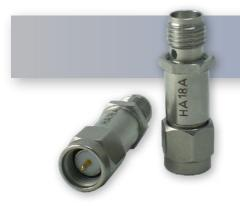
The HASCO Fixed Attenuator **HA18A-09** is rated to 2 Watts and operates from DC to 18GHz. The versatile coaxial package uses SMA male to SMA female connectors.
