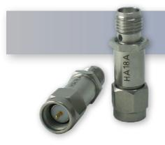
The HASCO Fixed Attenuator **HA18A-13** is rated to 2 Watts and operates from DC to 18GHz. The versatile coaxial package uses SMA male to SMA female connectors.
