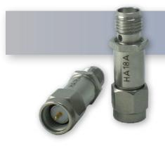
The HASCO Fixed Attenuator **HA18A-19** is rated to 2 Watts and operates from DC to 18GHz. The versatile coaxial package uses SMA male to SMA female connectors.
