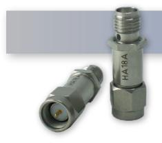
The HASCO Fixed Attenuator **HA18A-20** is rated to 2 Watts and operates from DC to 18GHz. The versatile coaxial package uses SMA male to SMA female connectors.
