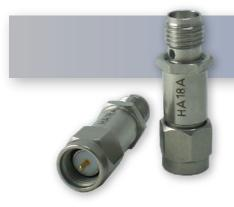
The HASCO Fixed Attenuator **HA18A-30** is rated to 2 Watts and operates from DC to 18GHz. The versatile coaxial package uses SMA male to SMA female connectors.
