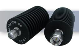
The HASCO Fixed Attenuator **HA18A10W-03** is rated to 10 Watts and operates from DC to 18GHz. The versatile coaxial package uses SMA male to SMA female connectors.
