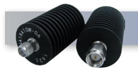
The HASCO Fixed Attenuator HA18A10W-15 is rated to 10 Watts and operates from DC to 18GHz. The versatile coaxial package uses SMA male to SMA female connectors.
