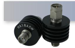
The HASCO **HA18A5W-.5** is an RF attenuator that operates from DC to 18 GHz and handles up to 5 Watts (CW). This attenuator is constructed with SMA Male to SMA Female connectors.
