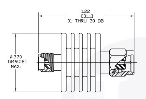
To view online, go to: 1 dB - fixed-attenuator-sma-male-to-sma-female-up-to-18-ghz-rated-to-5-watts-with-black-aluminum-heat-sink-body/
