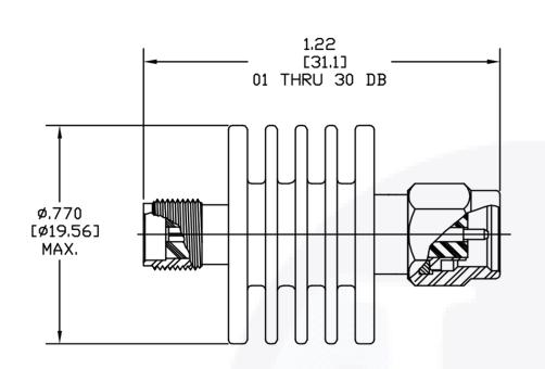
To view online, go to: 4 dB - fixed-attenuator-sma-male-to-sma-female-up-to-18-ghz-rated-to-5-watts-with-black-aluminum-heat-sink-body/
