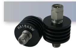
The HASCO **HA18A5W-10** is an RF attenuator that operates from DC to 18 GHz and handles up to 5 Watts (CW). This attenuator is constructed with SMA Male to SMA Female connectors.
