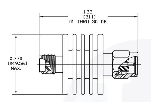
To view online, go to: 20 dB - fixed-attenuator-sma-male-to-sma-female-up-to-18-ghz-rated-to-5-watts-with-black-aluminum-heat-sink-body/
