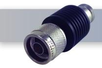
10 dB - Fixed Attenuator N Male To N Female Up To 18 GHz Rated To 10 Watts With Black Aluminum Heatsink Body
