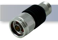
4 dB - Fixed Attenuator N Male To N Female Up To 18 GHz Rated To 5 Watts With Passivated Stainless Steel Body
