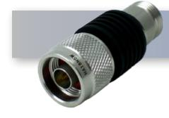
The HASCO Fixed Attenuator HA18N5W-05 is rated to 10 Watts and operates from DC to 18GHz. The versatile coaxial package uses N male to N female connectors.
