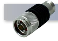
The HASCO Fixed Attenuator HA18N5W-07 is rated to 10 Watts and operates from DC to 18GHz. The versatile coaxial package uses N male to N female connectors.
