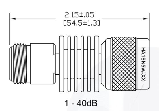
To view online, go to: <a href="https://www.hasco-inc.com/attenuators/20-db-fixed-attenuator-n-male-to-n-female-up-to-3-ghz-rated-to-5-watts-with-black-aluminum-heatsink-body/">https://www.hasco-inc.com/attenuators/20-db-fixed-attenuator-n-male-to-n-female-up-to-3-ghz-rated-to-5-watts-with-black-aluminum-heatsink-body/</a>
