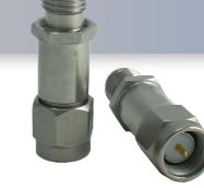
The HASCO Fixed Attenuator **HA26A-06** is rated to 2 Watts and operates from DC to 26 GHz. The versatile coaxial package uses SMA male to SMA female connectors.
