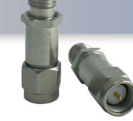
The HASCO Fixed Attenuator **HA26A-07** is rated to 2 Watts and operates from DC to 26 GHz. The versatile coaxial package uses SMA male to SMA female connectors.
