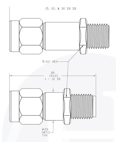
To view online, go to: <a href="https://www.hasco-inc.com/attenuators/ha26a-08-sma-male-to-female-attenuator-dc-26ghz-8db-with-hex-nut/">https://www.hasco-inc.com/attenuators/ha26a-08-sma-male-to-female-attenuator-dc-26ghz-8db-with-hex-nut/</a>
