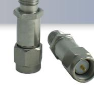
The HASCO Fixed Attenuator **HA26A-09** is rated to 2 Watts and operates from DC to 26 GHz. The versatile coaxial package uses SMA male to SMA female connectors.
