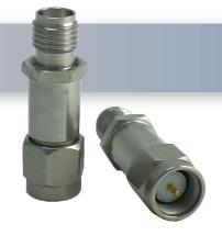
11 dB - Fixed Attenuator SMA Male To SMA Female Up To 26 GHz Rated To 2 Watts with Passivated Stainless Steel Body
