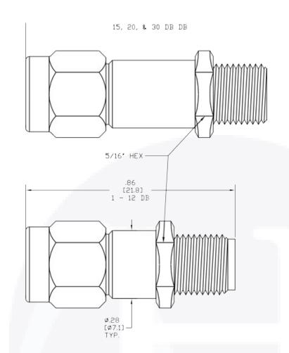
To view online, go to: <a href="https://www.hasco-inc.com/attenuators/ha26a-12-sma-male-to-female-attenuator-dc-26ghz-12db-with-hex-nut/">https://www.hasco-inc.com/attenuators/ha26a-12-sma-male-to-female-attenuator-dc-26ghz-12db-with-hex-nut/</a>
