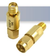
1 dB - Fixed Attenuator SMA Male To SMA Female Up To 3 GHz Rated To 2 Watts with Gold Plated Brass Body
