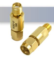
The HASCO Fixed Attenuator **HA3A2-02** is rated to 2 Watts and operates from DC to 3 GHz. The versatile coaxial package uses SMA male to SMA female connectors.
