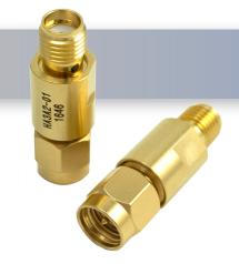
3 dB - Fixed Attenuator SMA Male To SMA Female Up To 3 GHz Rated To 2 Watts with Gold Plated Brass Body
