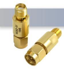
The HASCO Fixed Attenuator HA3A2-09 is rated to 2 Watts and operates from DC to 3 GHz. The versatile coaxial package uses SMA male to SMA female connectors.
