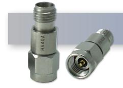
The HASCO Fixed Attenuator **HA40A-01** is rated to .5 Watts and operates from DC to 40 GHz. The versatile coaxial package uses 2.92 mm male to 2.92 mm female connectors.
