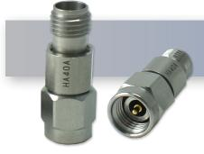
2 dB - Fixed Attenuator 2.92 mm Male To 2.92mm Female Up To 40 GHz Rated To .5 Watts with Passivated Stainless Steel Body
