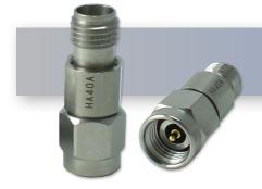
The HASCO Fixed Attenuator **HA40A-03** is rated to .5 Watts and operates from DC to 40 GHz. The versatile coaxial package uses 2.92 mm male to 2.92 mm female connectors.
