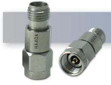
5 dB - Fixed Attenuator 2.92 mm Male To 2.92mm Female Up To 40 GHz Rated To .5 Watts with Passivated Stainless Steel Body
